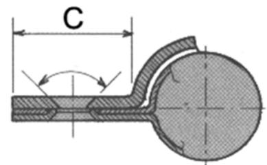
Liobex Single Action Hinges up to 6" are supplied in right hand configuration only, the capstan being at the top of the hinge. For left hand doors the capstan is set at the bottom. 7" and 8" are supplied handed and should be fitted accordingly with the capstan at the top in both instances.
